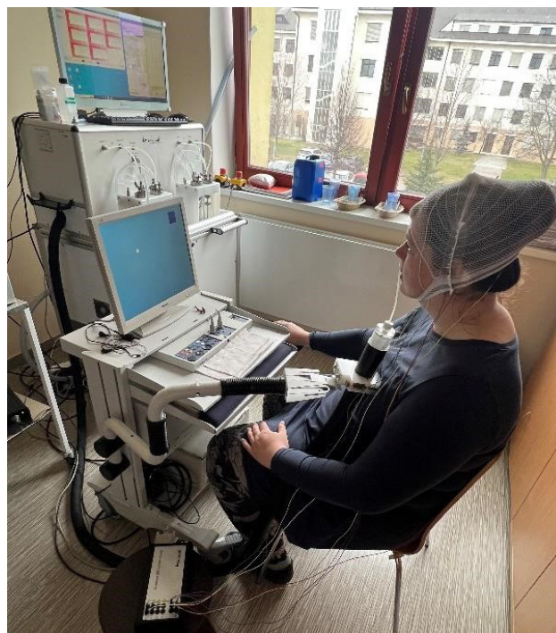
Fig. 1. Objective olfactometer OL 024 Burghart – measurement of olfactory event-related potentials (OERPs) (from corresponding author's archive).
