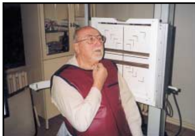
Fig. 3. A photograph showing an examined person wearing a protective apron and holding the acceleration recorder. The AKG C 10005 microphone with the MZ-R3 mini-disc was located approx. 1m from the person. The recording device did not include a secondary diaphragm and the focus – camera distance was about 1.2 m.
