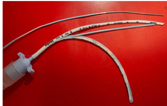
Fig. 3. The ruptured piece of plastic coat can be seen inside the snipped endotracheal tube (Portex I.D. 2.5 mm). This inside part of the plastic coat has its original width (left side) in comparison with two thinner parts of the overstretched plastic coat interrupted by the thinnest part (right side) that remains on the wire of the stylet (Sheridan/Sher-I-Slip, HUDSON RCI, O.D. 1.7 mm).
