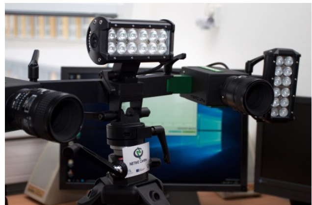
Fig. 5. Mercury RT optical device for measuring deformities.
