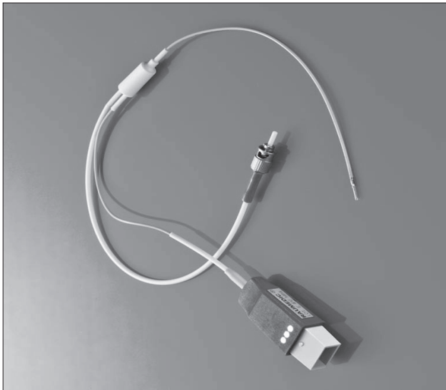
Fig. 1. Multiparametric sensor Neurovent® PTO (Raumedic AG, Germany).
